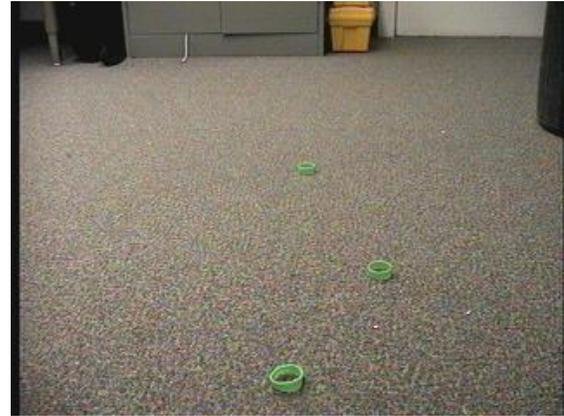
**Figure 2.** A robot's eye view of several of the rings which were used as landmarks. During an experimental run, they are deployed about three meters apart.
