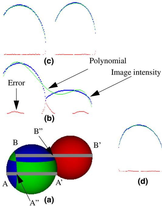
**Figure 5: (a) Test image, (b) fitting one polynomial to B-B', (c) fitting two polynomials to B-B', (d) fitting one polynomial to A-A'. In (b), (c), and (d), the bottom line shows the error in the fit, while the top two lines show the image intensity overlaid by the least-squares polynomial.**
